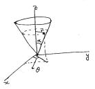
A particle of mass m is constrained to move on the inside surface of a smooth cone of half-angle  $\alpha$  (see figure). The particle is subject to gravitational force.
